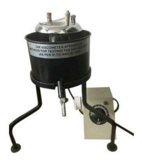
Tar Viscometer apparatus
